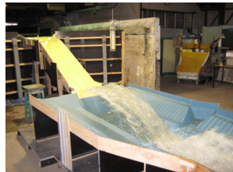
Physical model of a spillway chute plunge pool
