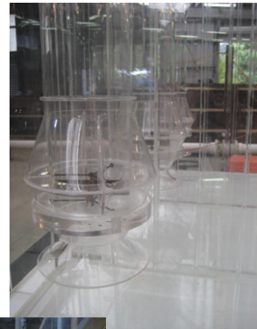
Bellmouth pump intake pipes
