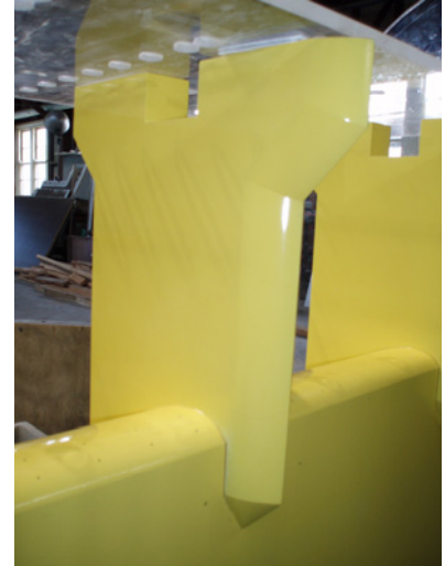
Proposed pier nose design
